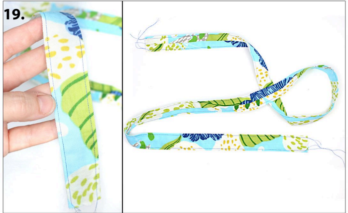
Step 19. Edgestitch to finish along both long edges of the Strap (B). Set aside.
